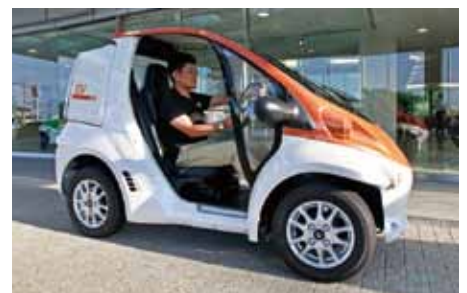
Super-small EV Coms developed and sold by Toyota Auto Body. It can be charged via standard 100 VAC electrical outlet.
