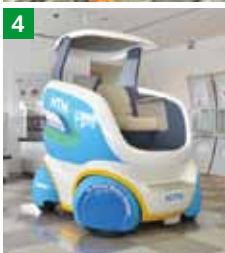
4 NTN, a major ball bearing manufacturer, developed an in-wheel motor. The experimental car can change directions while stationary.
