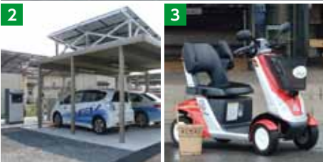
1 Ryusei Kaikan roadside station has two chargers. Solar panels decrease operating costs. 2 A park-and-ride project is being tested through February 2014 at Kagohara Station. The parking lot uses solar power and features a new storage battery. 3 At the Chichibu Cemetery, Honda's rental electric cart Monparu is available for seniors and is garnering favorable attention.
