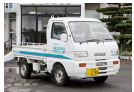
Converted light truck-EV developed by Tohoku Jidosha in Hachinohe City.
