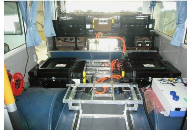
バッテリ搭載 Cabin rear battery installation
