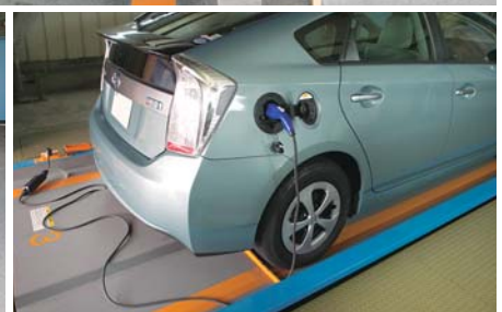
Electrical power sockets are located to the front and rear of the parking palettes. Charging starts automatically after connecting the charging cable and parking the car, and is provided at no charge. The association aims to expand the usage of EV car sharing to local citizens as well.
