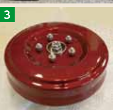
1 OVEC-ONE, based on Mitsubishi Motors' GALANT FORTIS. 2 OVEC director Hiroshi Yoshida, who spearheaded development. 3 Thin, in-wheel motors separately control each of the four wheels.
