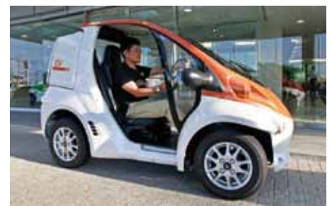
Super-small EV Coms developed and sold by Toyota Auto Body. It can be charged via standard 100 VAC electrical outlet.
