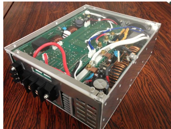
"Single Switch Converter Type Charging Unit (Prototype)" (Isahaya Electronics)
