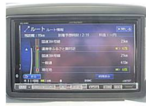
Downloading "My PLAN" from ITS spot (IP) to Car-Navi makes possible to set the destination smoothly
