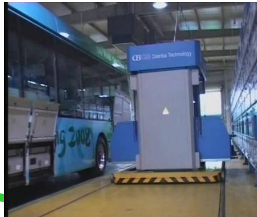
Charging and Swap station
